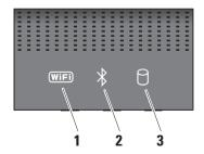
1 WiFi status light – Turns on when wireless networking is enabled.
